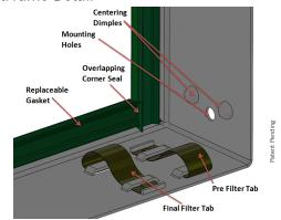
Compression tabs securely hold filters in place without the use of cumbersome fasteners. Premium gasket ensures all air moving through the system is treated by the air filter. There are three mounting holes on the vertical and two on the horizontal to provide a secure frame-to-frame assembly.
